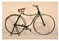
The bicycle featured two wheels of the same size and a chain drive to the rear wheel.
